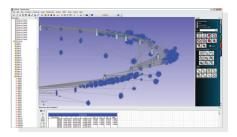
A powerful feature that leverages the uncertainty characteristics of different instruments to provide a much more accurate instrument network than that of traditional alignment methods.
